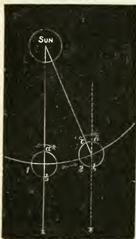
Fig. 31.—Diagram showing how the difference between the lengths of the Sidereal and Mean day arises.
